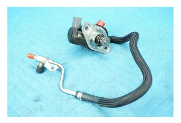
64. The fuel rails and high-pressure fuel pump are located in the rear of the engine compartment. Here, the high-pressure fuel pump has two fuel line connections. A braided low-pressure fuel line hose comes into the fuel pump (the "braided hose"), and a hard fuel line leads out to the fuel rail. Together, these constitute the "upper connection." Below is a picture depicting the location of the high-pressure fuel pump within the engine compartment:
